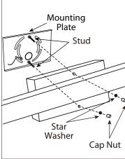
1 o Remove the mounting plate from the fixture by unscrewing the cap nuts and star washers.
