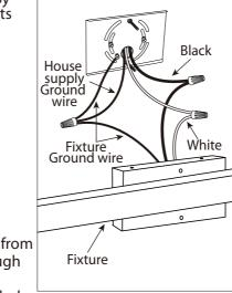
2. Feed power cords from the electrical box through the centre hole of the mounting plate. Align holes of mounting plate over electrical box and secure with electrical box screws (not included).
